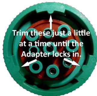
Note, the Adapter's locking mechanism is designed to be used in heavy duty vehicles such as highway trucks and construction equipment and can be very tight to lock. To ease locking and unlocking your Adapter, you can trim away the lower half of the three nipples located on the inside of the ring (see picture above). Be careful that you don't trim too much of the nipples otherwise the Adapter will not lock, in which case you will need to replace the locking ring.
